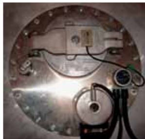
Weight and measures approved manhole with overfill prevention sensor and SCS Open/Close sensor
