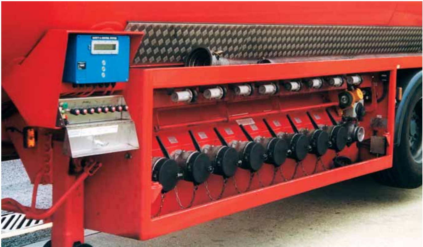
SCS system with user-friendly display up to 12 compartments
